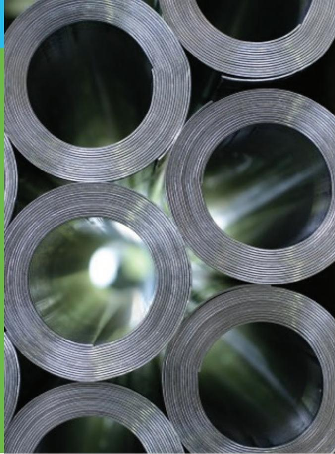
**Lead sheet, is used in the construction industry for roofing and as a radiation shield in the healthcare industry and has an impressive recycling record – all lead sheet is manufactured from recycled material, and more than 95% is collected and recycled.**
